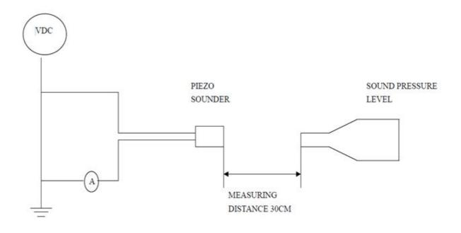
MIC: S.P.L meter TES1351B or equivalent
