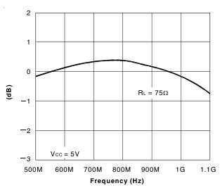
Insertion Loss vs. Frequency
