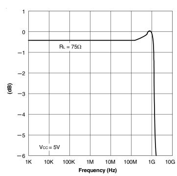
Insertion Loss vs. Frequency
