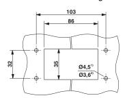
Panel cutout <sup>2)</sup> When self-tapping screws are used (Torx® 20, M4)
